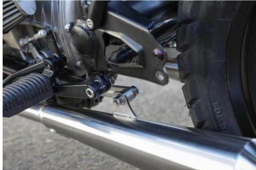
7. Align the exhaust system and tighten all screws connections, starting from the outlet, of the exhaust system from front to back, so everything is in line
